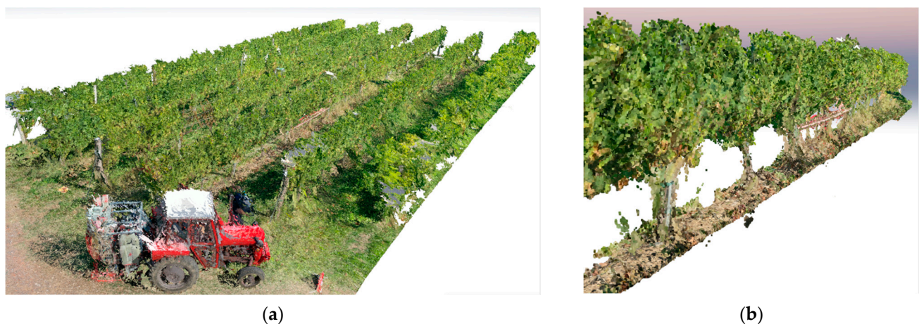
Figure 6. The UAS surveyed experimental vineyard as a point cloud from UAS photogrammetry measurements with about 195 million points (a), and the section used for the method comparison with about 30 million points (b).
