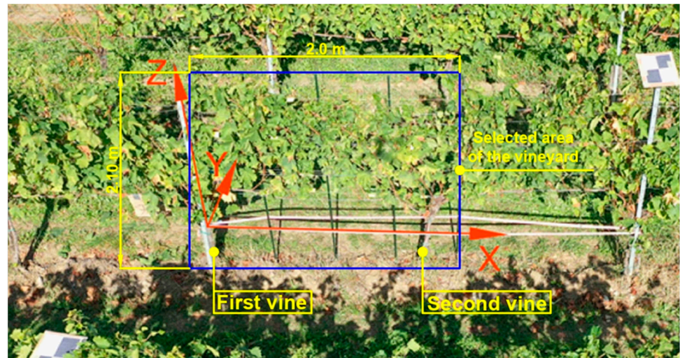
Figure 4. A (blue) section of the vineyard used for manual defoliation measurements, with local coordinate system ( X , Y , Z ). The green vertical poles and the red ribbon (collinear with x ) can be seen; the horizontal ropes were somewhat hidden by the leaves.
