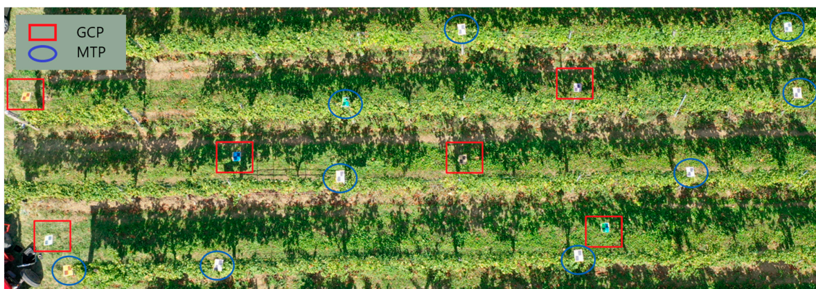
Figure 2. Lidar and UAS survey area 28 m × 7 m (4 vine rows) and the distribution of GCPs and MTPs. The GCPs were fixed on the ground between the vine rows and the MTPs were fixed at the top of the vine rows.
