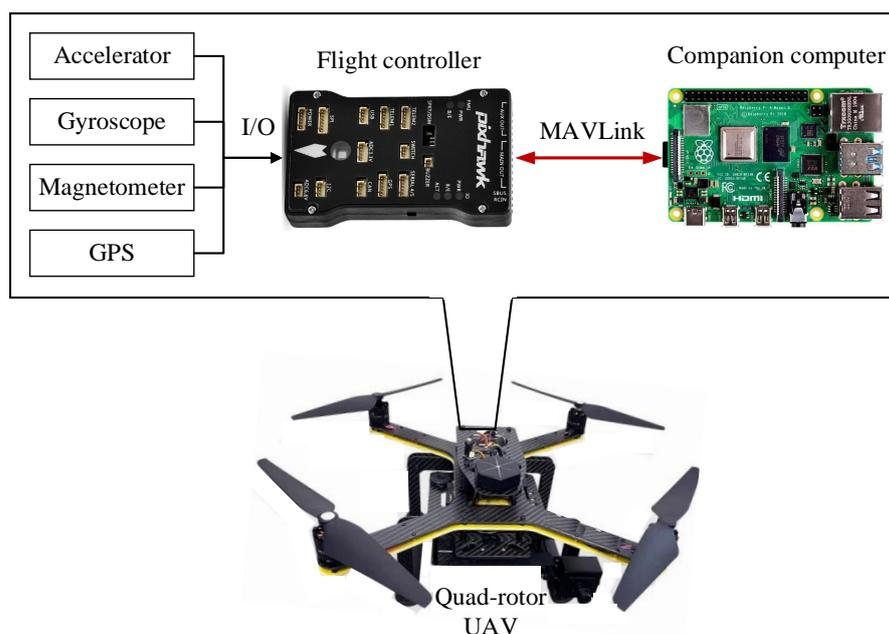
**Figure 4.** The structure of our UAV
