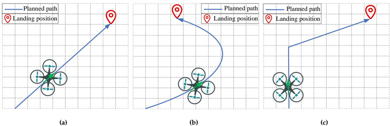
**Figure 5.** Flight paths. (a) Straight line path; (b) Curved line path; (c) Turning path.
