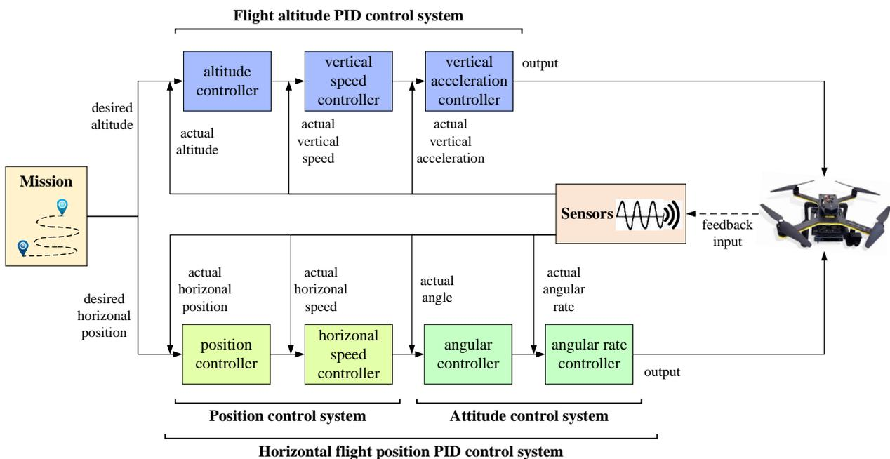
**Figure 2.** A UAV PID control system.
