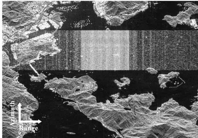
**Figure 9.** Jamming result of the designed NLFM waveform.
