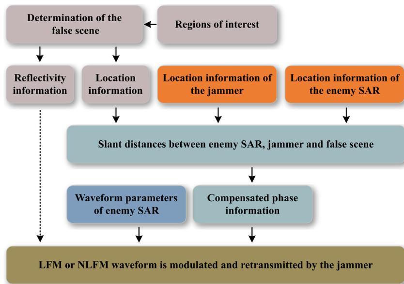
Figure 7. Flowchart of barrage jamming.
