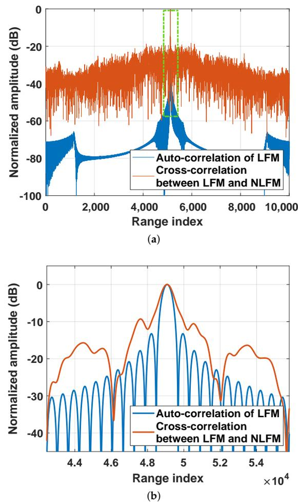
**Figure 3.** Comparison between LFM waveform and the designed NLFM waveform. (a) Autocorrelation and cross-correlation functions; (b) enlarging and upsampling result of the area marked by the rectangle in (a).
