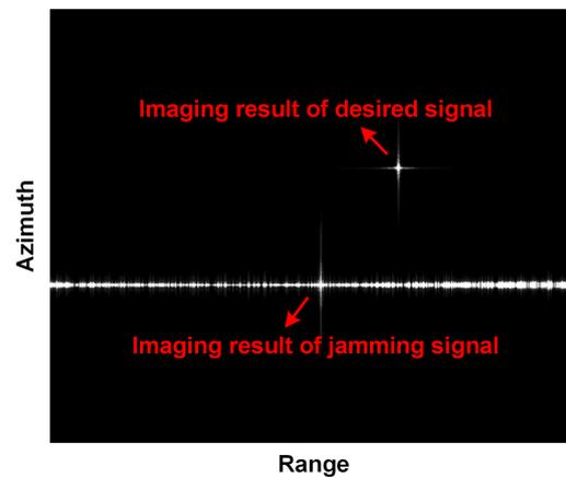
Figure 4. Imaging result of point targets.
