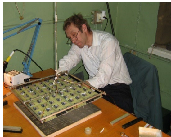
Figure 3. 16 \times 16 element planar antenna array designed at JSC Jupiter-Z.
