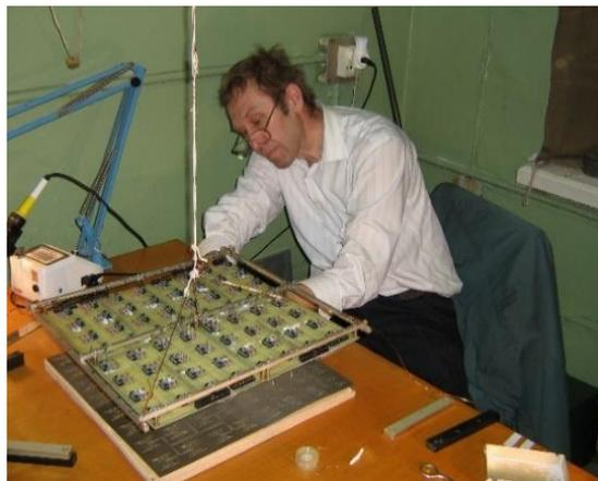
**Figure 3.** 16 × 16 element planar antenna array designed at JSC Jupiter-Z.
