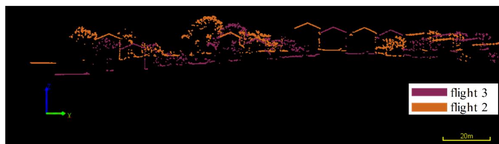
Figure 22. Vertical section of point cloud in opposing flight strips (flight 2 and flight 3) without installation angle compensation.
