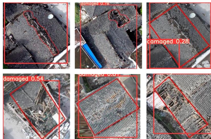
**Figure 16.** The samples for UAV images of different types of houses damaged by the Ya'an Ms7.0 earthquake on 20 April. The red vertical bounding boxes are the results of our method. The red irregular polygons are the annotations from references [8,9].
