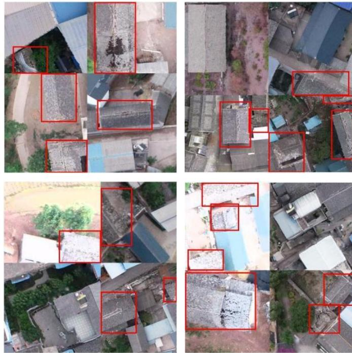
**Figure 7.** Examples of Mosaic data enhancement. Mosaic scales the four different images and arranges them to fit in the desired output size. The red boxes are the bounding boxes for damaged houses.
