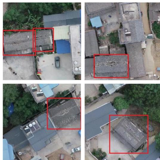
**Figure 5.** The samples of damaged houses by the Yangbi Earthquake. The red boxes are the bounding boxes for damaged houses.
