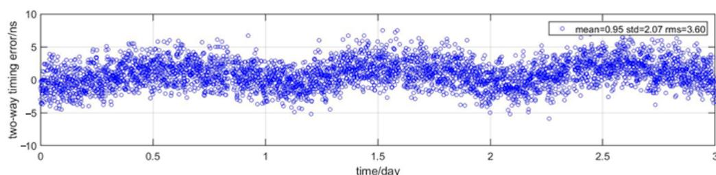
**Figure 10.** RDSS two-way timing accuracy (orbit maneuver state).
