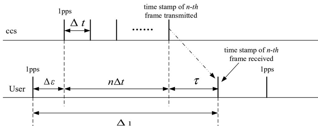
Figure 1. The one-way timing principle.
