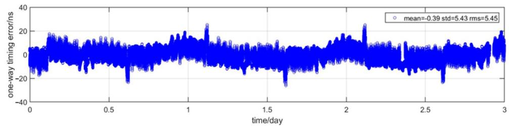
**Figure 3.** RDSS one-way time service error (normal state).
