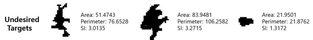
Figure 10. Morphology characteristics of undesired targets.
