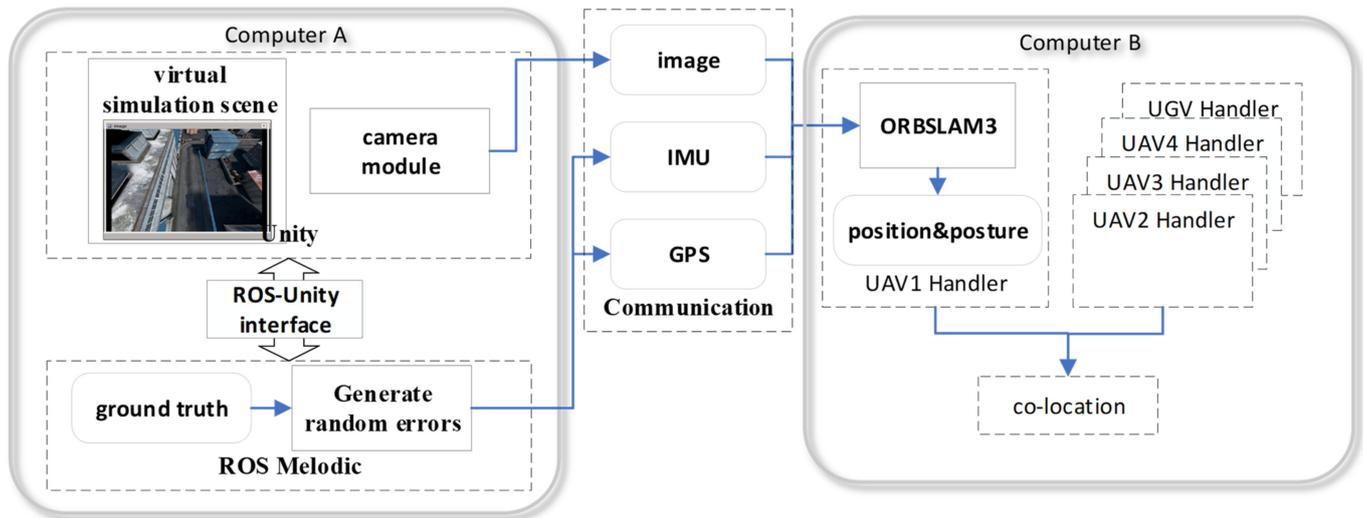
**Figure 5.** The virtual data generation program is deployed on Computer A, and the agent handler and cooperative location program is deployed on Computer B. They are connected using a gigabit network.
