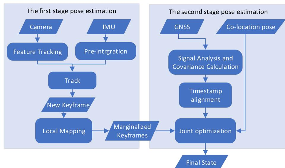
**Figure 3.** The tracking thread processes sensor information in real time and initially estimates the pose of the current frame. In the process of tracking the local map, the track thread determines whether the current frame is used as a keyframe. Different from ORBSLAM3's keyframe addition strategy, when valid GNSS positioning information completes timestamp alignment, frames aligned with GNSS information are also inserted as keyframes.
