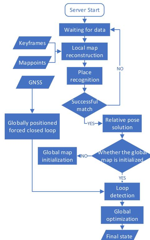
**Figure 2.** The running process of the co-location module in Figure 1 is explained in detail. The function
