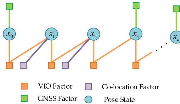
**Figure 4.** Schematic diagram of the pose graph structure to be optimized in the second stage. The circle is the state quantity, and the yellow square is the constraint of local observation, that is, the relative pose transformation of VIO from ORBSLAM3. The other colored squares are constrained by global observations.
