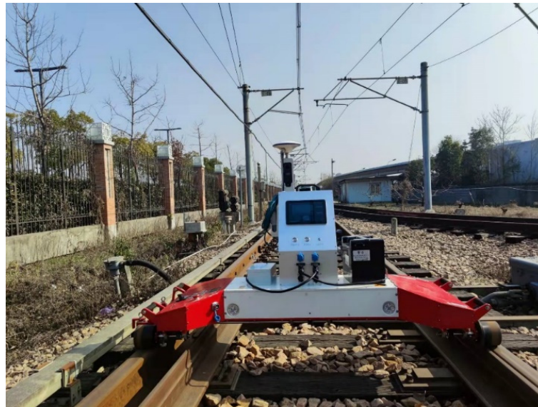
Figure 11. Mobile laser scanning system in experiment environment.
