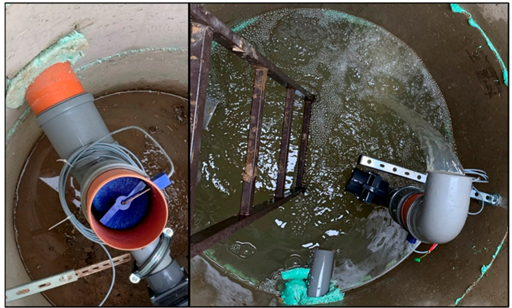
Figure 3. Fixed WLCS installed in the manhole with propeller flow meter (left) and water overflow after a rainfall-runoff event on 14 May 2021.
