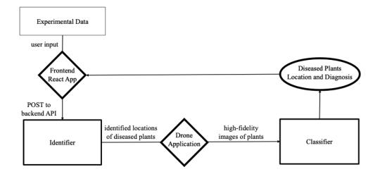
Figure 3. The pipeline with identifier and classifier.
