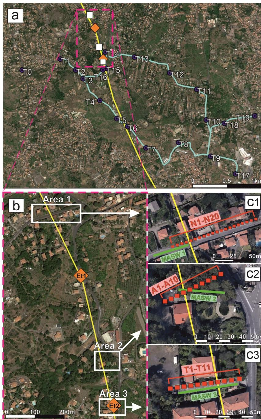
**Figure 2.** (a) Map of the levelling route (sky-blue line) across the Trecastagni Fault (TF). Blue circles indicate the levelling benchmarks; orange diamonds indicate the position of the extensometers. White squares indicate the location of seismic surveys. (b) Yellow line indicates the TF, and the
