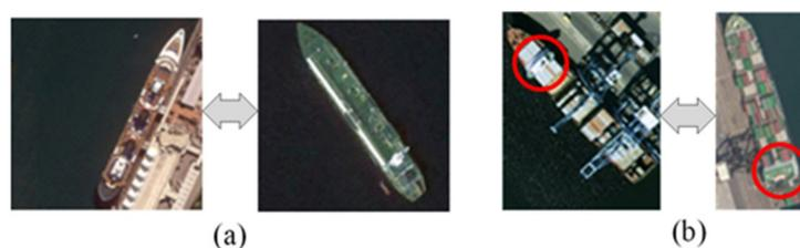
**Figure 1.** (a) Inter-class similarity, take ocean liner and ferry boat for example. (b) Intra-class differences, taking different container ships as an example, the position of the bridge is marked with red circles.
