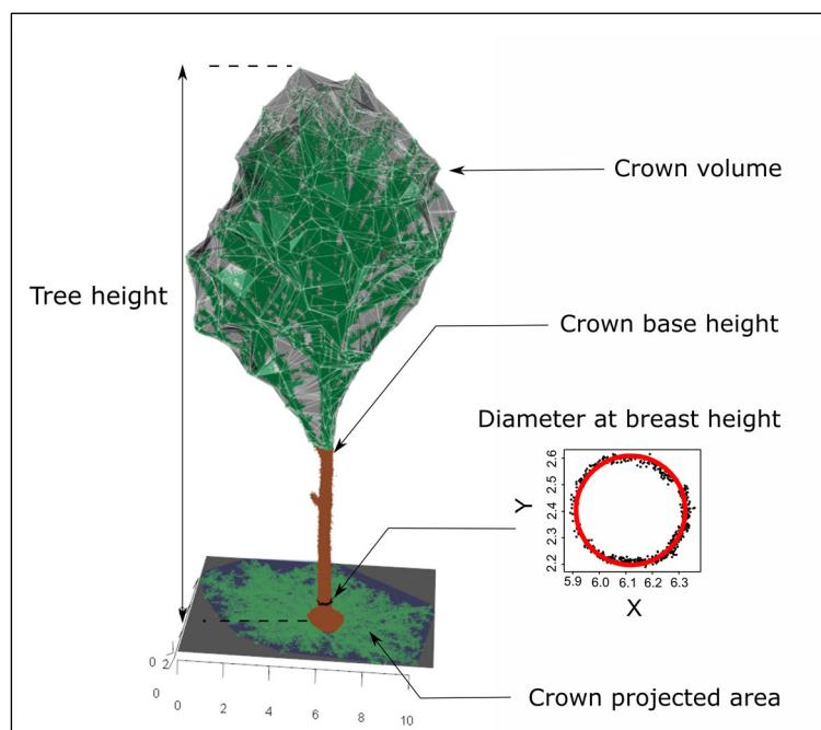
**Figure 5.** Tree structural attributes estimation from a MLS tree: tree height (H), crown base height (CBH), crown projected area (CPA), crown volume (CV), and diameter at breast height (DBH), estimated from a 5 cm slice of the stem at 1.3 m above the ground.
