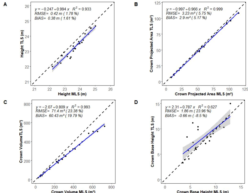
**Figure 7.** Comparison of (A) tree height (H); (B) crown projected area (CPA); (C) crown volume (CV) and (D) crown base height (CBH) for the 26 TLS and MLS trees. The blue line represents the linear regression. The grey zone is the 95% confidence band for predictions. The dashed black line represents the 1:1 line.
