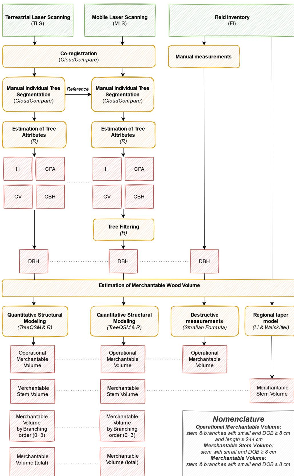
**Figure 3.** Overall data processing workflow for TLS, MLS, and field measurements (green: input; orange: processing; red: output; italic: software and formula). Acronyms: height (H), crown projected area (CPA), crown volume (CV), crown base height CBH), diameter at breast height (DBH), and diameter outside bark (DOB).
