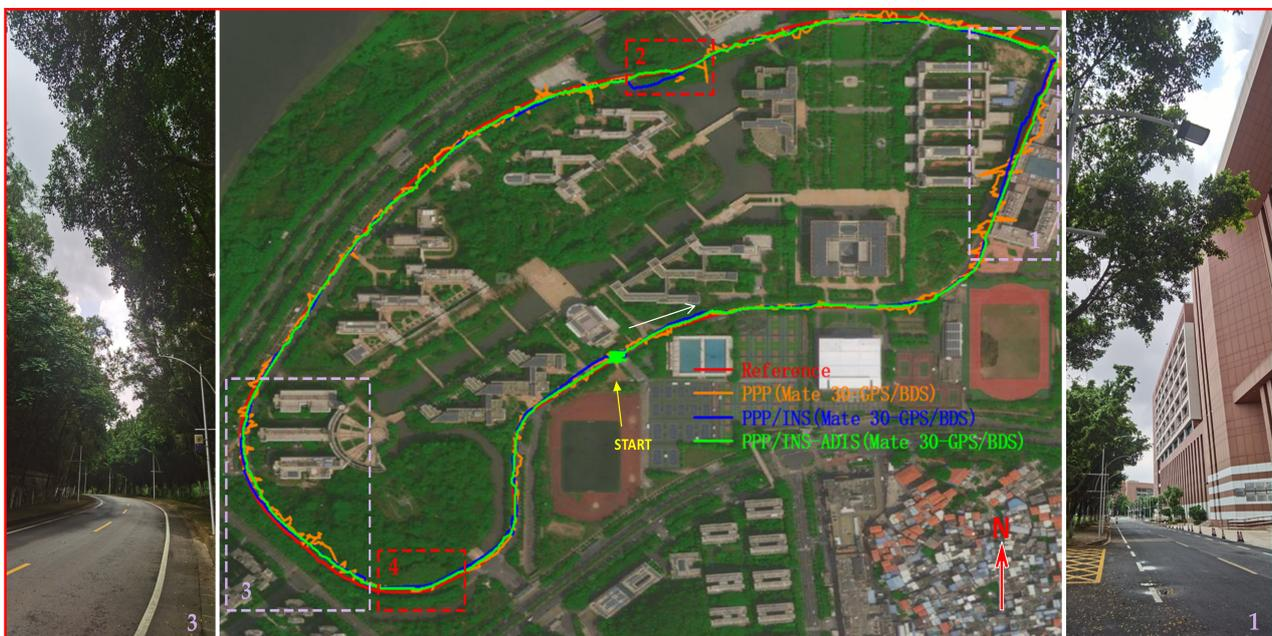
**Figure 16.** The long trajectories of GPS/BDS PPP, PPP/INS, and PPP/INS–ADIS solutions using Huawei Mate 30 and ADIS16405. Left: the realistic environment marked in the purple box 3. Right: the realistic environment marked in the purple box 1. The areas where the number of satellites cannot meet the requirements of GNSS positioning are marked by red boxes 2 and 4.
