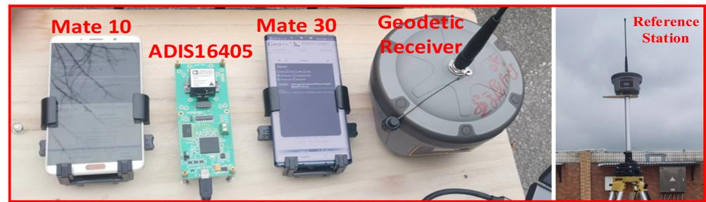
**Figure 1.** View of the experiment devices. Left: Huawei Mate 10, triaxial inertial sensor ADIS16405, Huawei Mate 30, and South geodetic receiver. Right: the reference station is placed in the open area on the roof.
