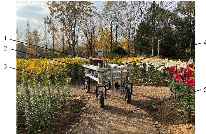
**Figure 11.** Experimental environment. 1. PC; 2. experimental platform; 3. flowers; 4. Intel RealSense D435i; and 5. unstructured path.
