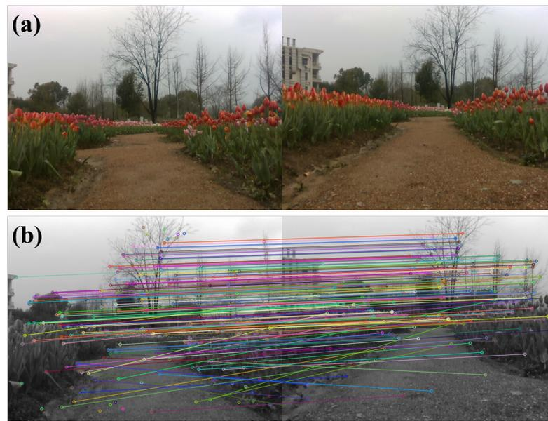
**Figure 8.** Feature rough matching. (a) Matching image; (b) results of feature matching.
