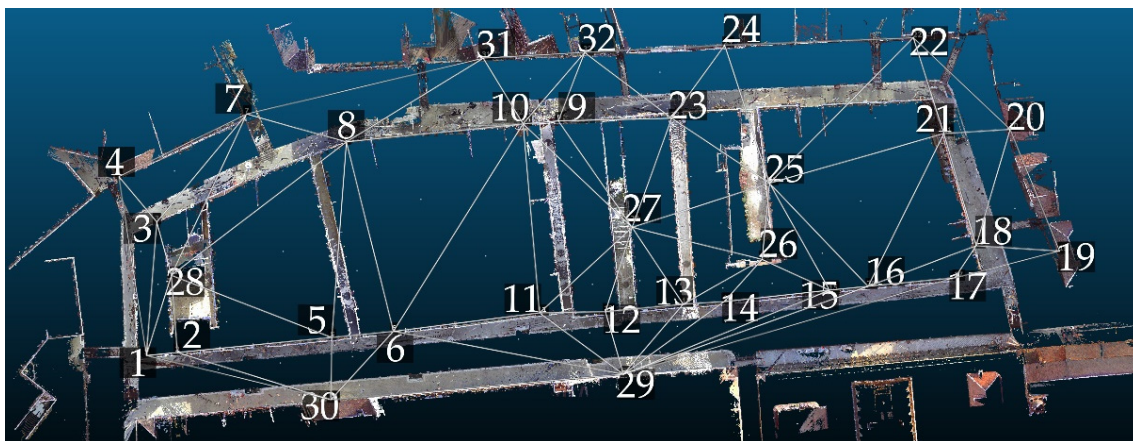
Figure 10. TLS control points and triangulation.
