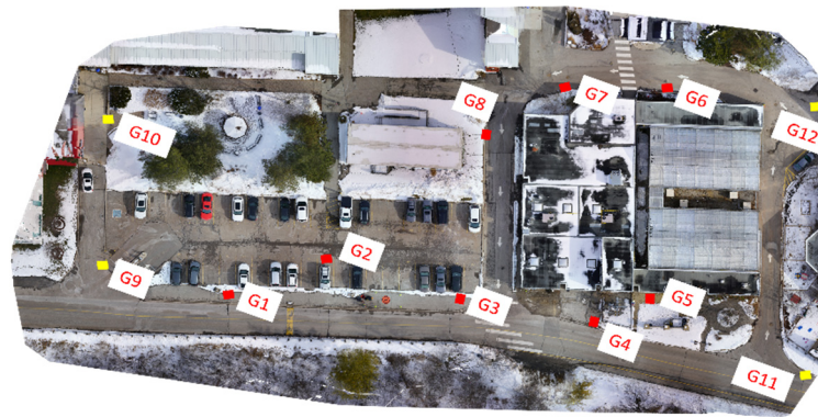
Figure 4. First study area with red and yellow squares highlighting the GCP positions. G1 through G12 represent the ground control points (GCPs) and check points.
