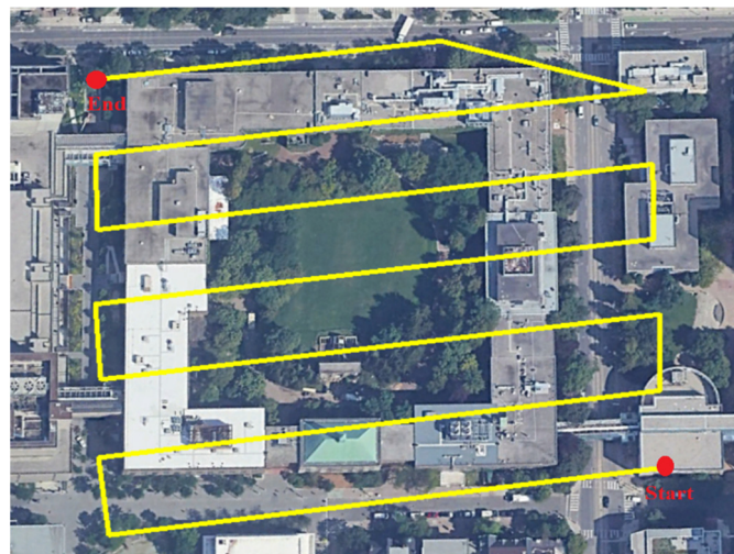
Figure 5. UAS flight lines above the second test site.
