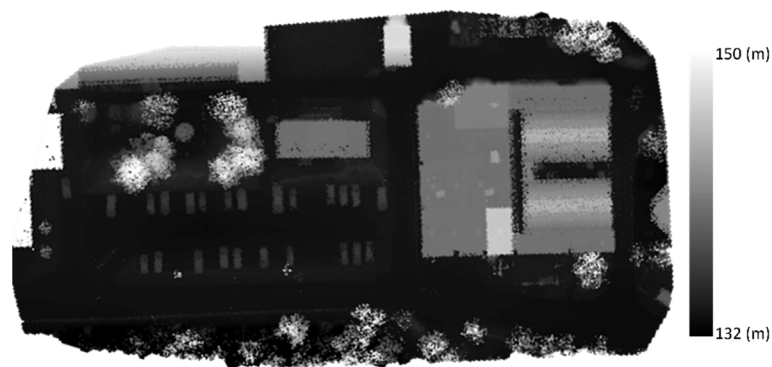
Figure 11. DSM raster generated using the LiDAR data point cloud for the first test site.
