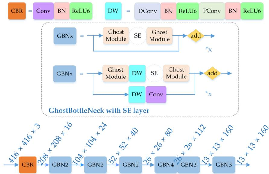
**Figure 7.** Diagram of GhostNet structure without fully connected layers. The ReLU activation function is used in Ghost Module. The symbol “\*x” indicates the GBNx is composed of x GBN structures.
