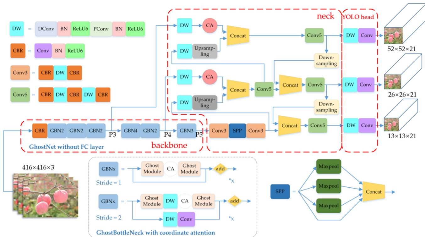
**Figure 4.** Improved YOLOv4 network. The Ghost Module in the backbone uses the ReLU activation function, while the rest of the network structures use the ReLU6 activation function. CA module means Coordinate Attention. The CA module in GhostBottleNeck is only present in the GBN structures at layers 4, 5, 10, 11, 12, and 14. The symbol “\*x” indicates the GBNx is composed of x GBN structures.
