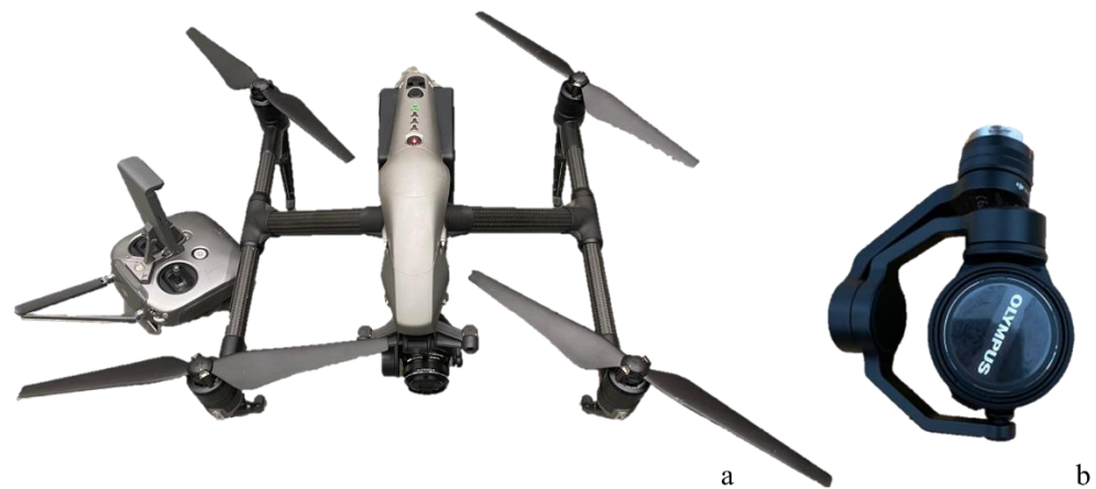
Figure 5. DJI Inspire II UAS: (a) DJI Inspire II drone, (b) DJI Zenmuse X5S camera and an Olympus M.Zuiko lens.
