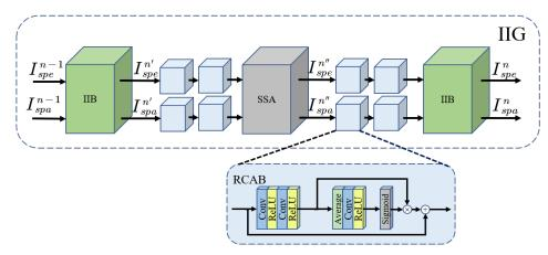
**Figure 2.** Schematic diagram of the information interaction group, " $\oplus$ " denotes elementwise addition, and " $\otimes$ " denotes matrix multiplication.
