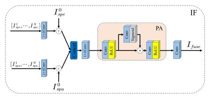
**Figure 5.** Schematic diagram of the information fusion module, " $\oplus$ " denotes elementwise addition, and " $\otimes$ " denotes matrix multiplication.
