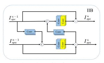
**Figure 3.** Schematic diagram of the information interaction block, " $\oplus$ " denotes elementwise addition, and " $\otimes$ " denotes matrix multiplication.
