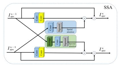
**Figure 4.** Schematic diagram of the spectral-spatial attention module, " $\oplus$ " denotes elementwise addition, and " $\otimes$ " denotes matrix multiplication.
