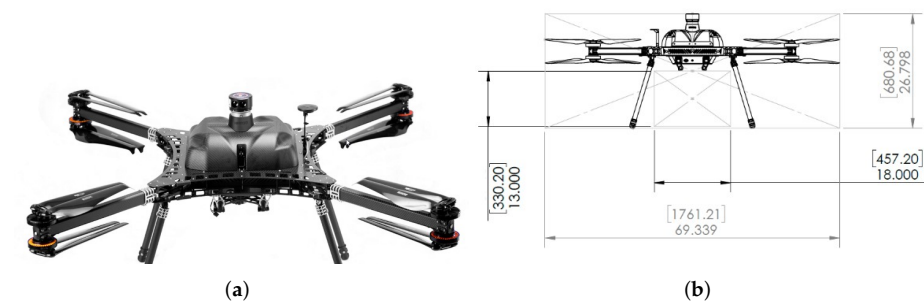
Figure 3. UAS platform. (a) Harris Aerial HX8. (b) HX8 dimensions.
