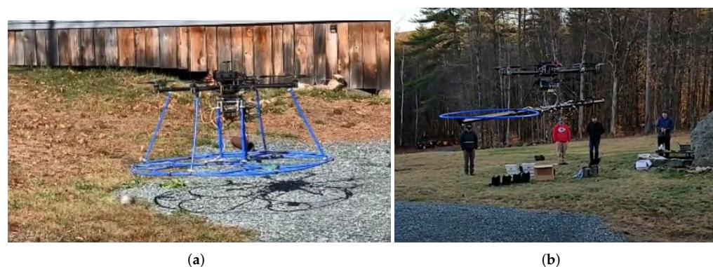
Figure 1. Previous UAS-mounted remote sensing systems. (a) UXO detection system. (b) Soil conductivity detection system.
