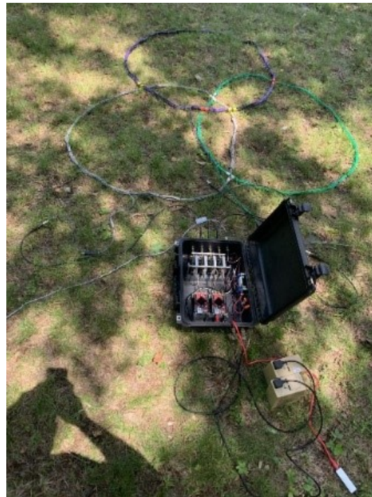
Figure 12. Sensor and dipole transmitter. (a) Block diagram of gradiometer sensor. (b) Simultaneous vertical magnetic dipole transmitter.
