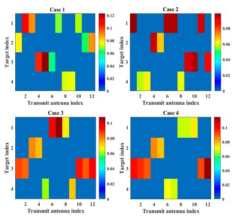
Figure 5. Transmit antenna selection and power allocation results under four cases.
