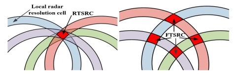
Figure 3. Target detection mechanism under range deception jamming.
