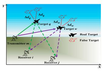
Figure 2. Intuitive process of multi-target detection under self-defense range deception jamming.
