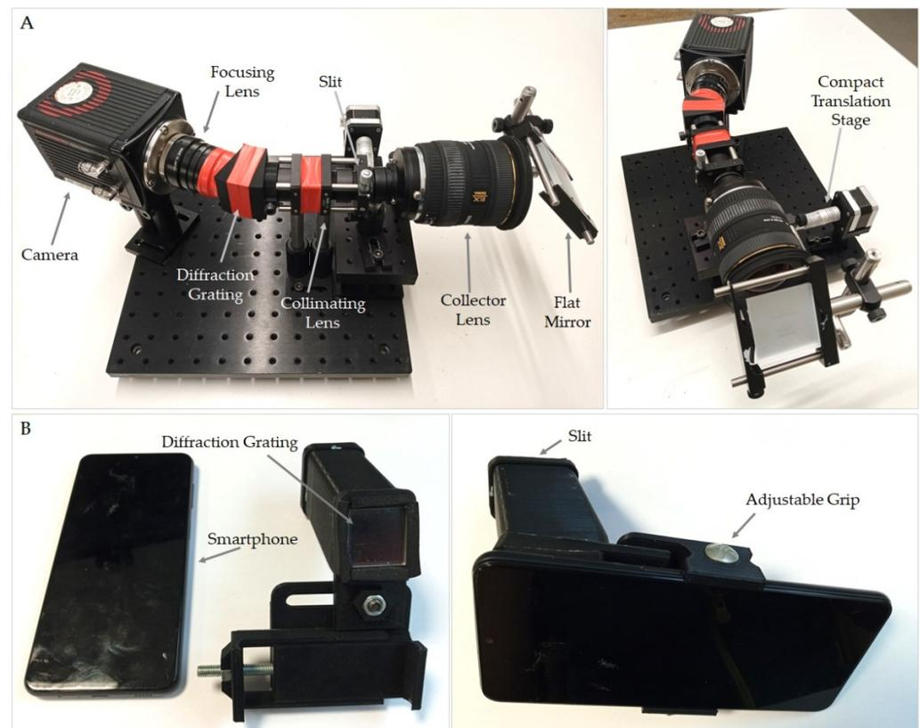
**Figure 1.** Low-cost hyperspectral imaging instrumentation utilised within this research. (A) shows the semi-portable Low-Cost High-Resolution instrument. (B) shows the ultra-low-cost Hyperspectral Smartphone instrument both before connection with a smartphone (left) and after connection and alignment of the spectral components with the built-in smartphone camera optics.
