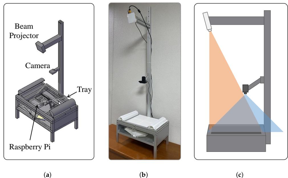
**Figure 5.** Local hardware device. (a) Cad design of the local device. (b) Photo of the local device. (c) Configuration of the camera and beam projector.
