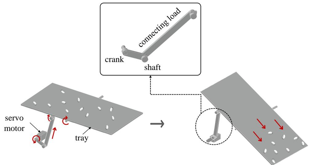
**Figure 6.** Motor system.
