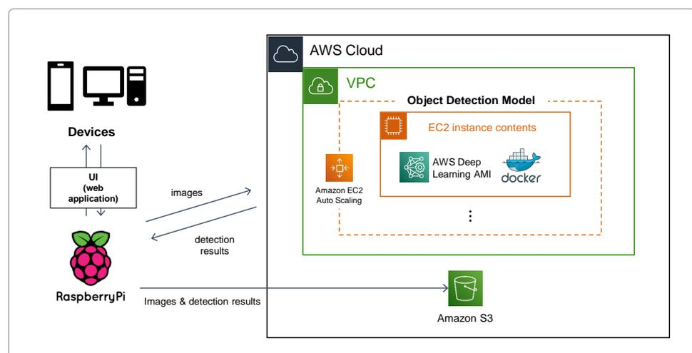
**Figure 4.** Object-detection server architecture based on AWS development stacks.
