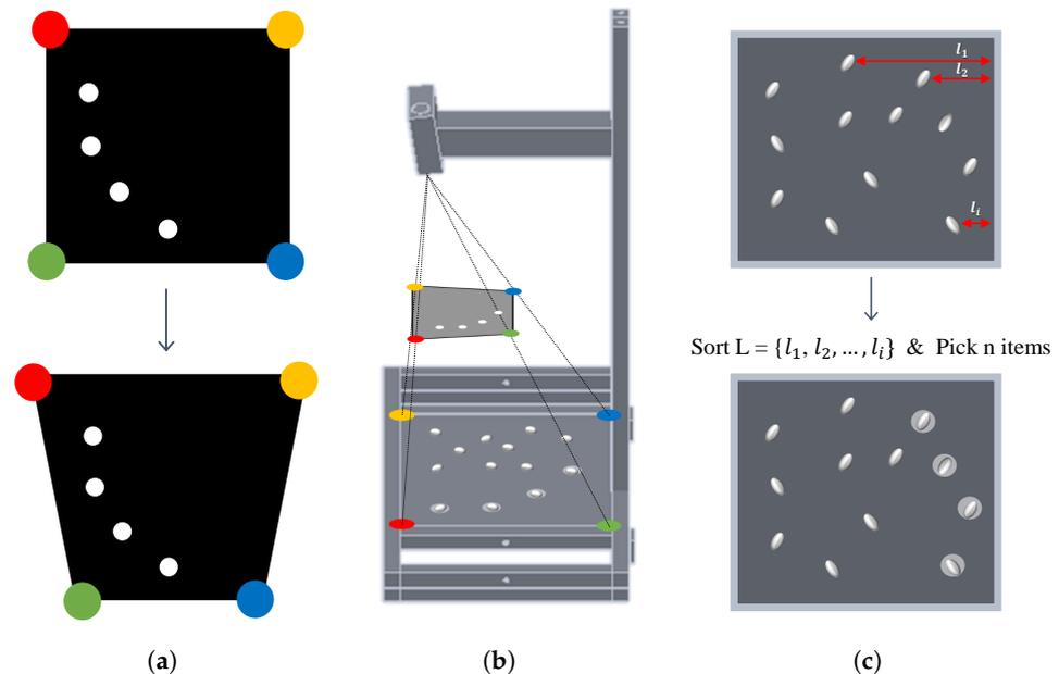
**Figure 7.** Beam projector output transformation. (a) Perspective transformation. (b) Transformed output from beam projector. (c) Process of selecting excessive items.
