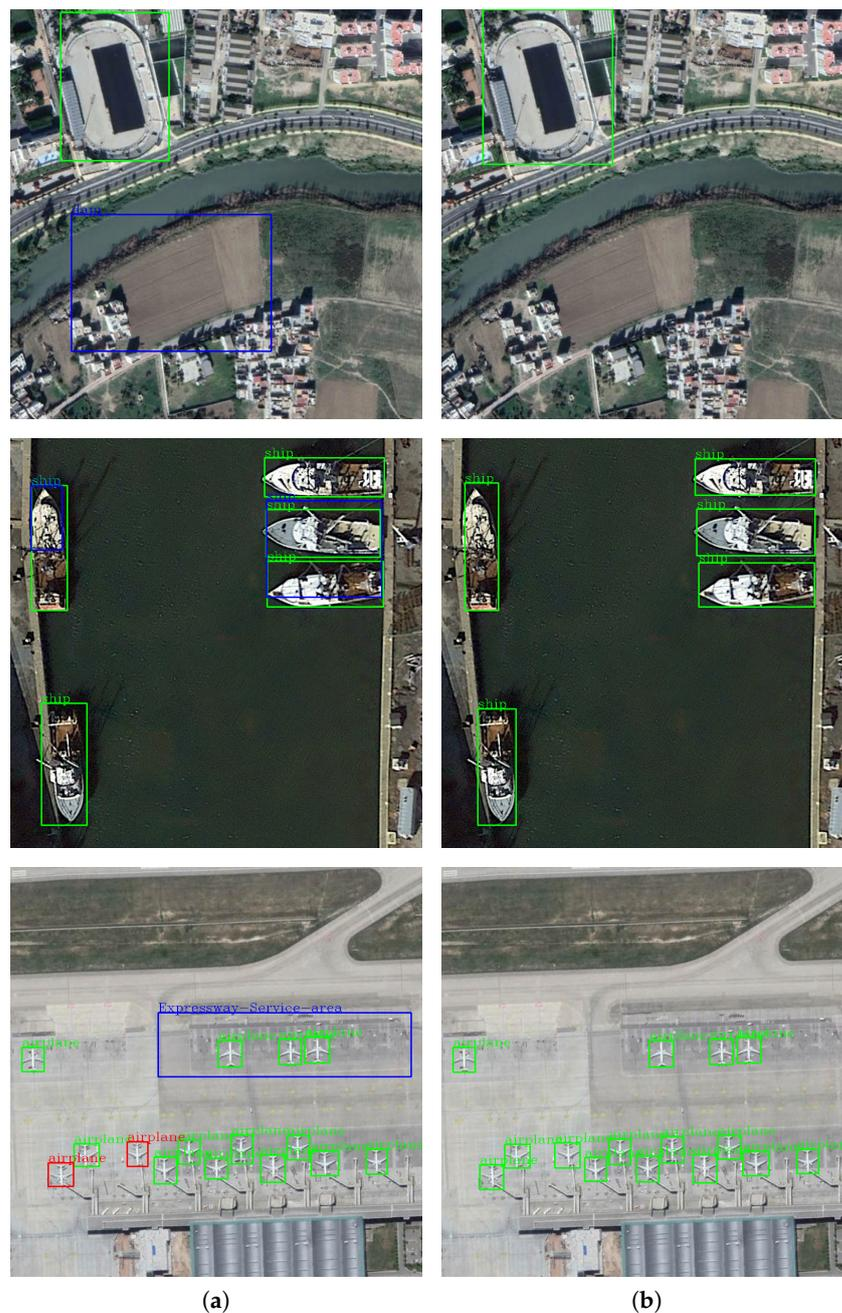
**Figure 7.** Some detection results comparison between FPN and the proposed method. (a) prediction of FPN; (b) prediction of the proposed method. The green, blue, and red rectangles represent TPs, FPs, and FNs, respectively.
