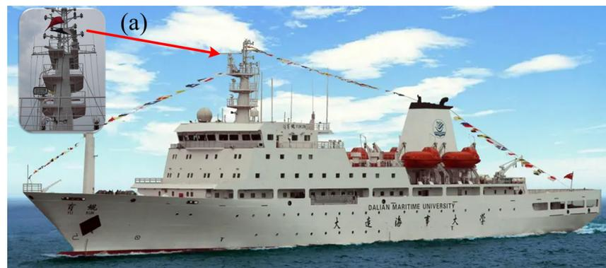
Figure 2. The experimental data acquisition platform. (a) The shipborne radar installation position.
