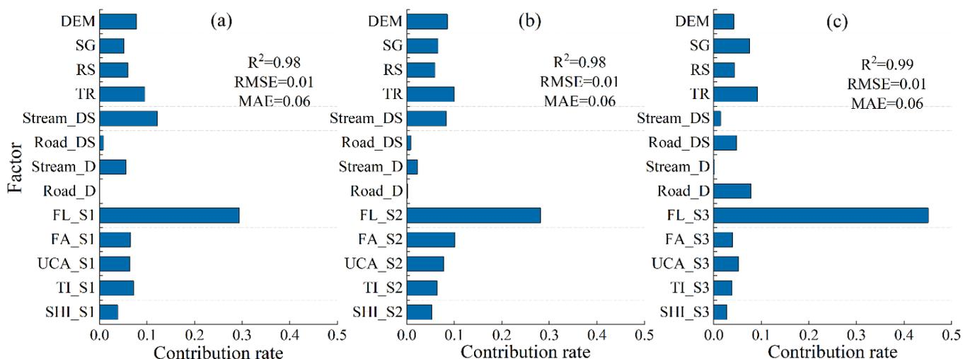
**Figure 7.** Contribution of influencing factors to sediment connectivity in scenarios S1 (a), S2 (b), and S3 (c). DEM, Digital Elevation Model; SG, slope gradient; TR, terrain relief; stream\_DS, distance to stream; Road\_DS, distance to road; stream\_D, stream density; Road\_D, road density; FL, flow length; FA, flow accumulation; UCA, upslope contributing area; TI, topographic index; SHI, Shimbil index.
