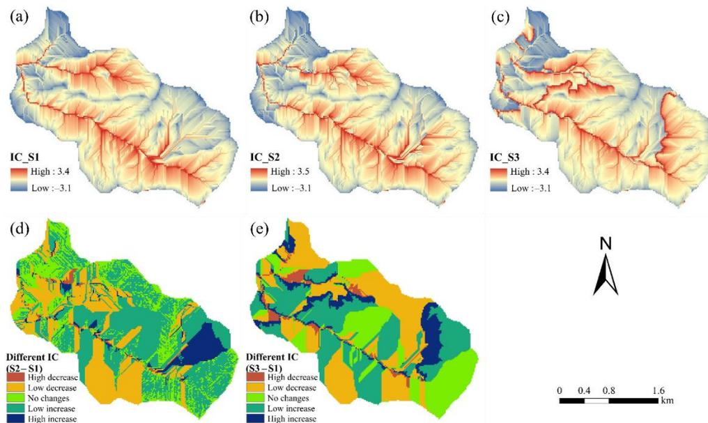
**Figure 5.** Spatial distribution of sediment connectivity under scenarios of S1 (a), S2 (b), and S3 (c), and changes in sediment connectivity in scenarios S2 (d) and S3 (e) compared to scenario S1.
