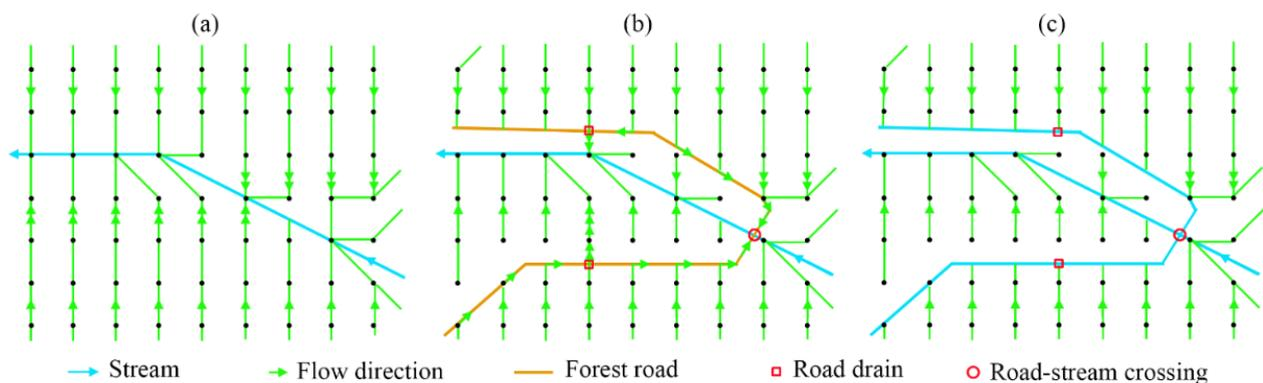
**Figure 2.** Schematic diagram showing the natural and altered direction and converging pathways of flow and sediment in scenarios S1 (a), S2 (b), and S3 (c).
