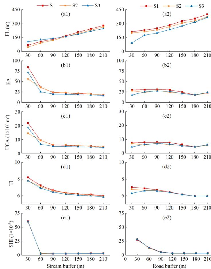
**Figure 4.** Variation in flow length (FL, **a1,a2**), flow accumulation (FA, **b1,b2**), upslope contributing area (UCA, **c1,c2**), topographic index (TI, **d1,d2**), and Shimbel index (SHI, **e1,e2**) with distance from stream and road in scenarios S1, S2, and S3.
