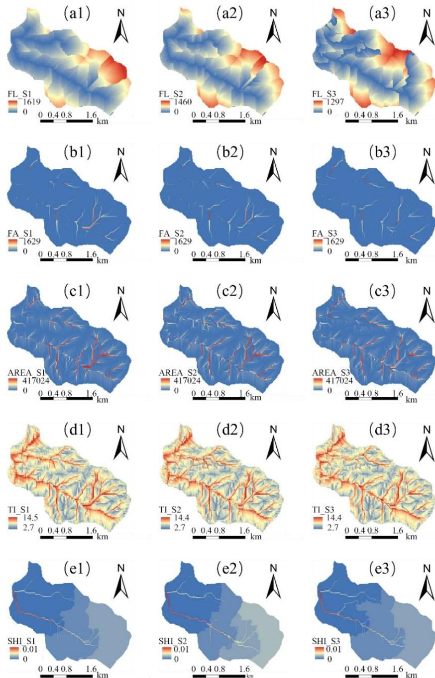
**Figure 3.** Spatial distribution of flow length (a1–a3), flow accumulation (b1–b3), upslope contributing area (c1–c3), topographic index (d1–d3), and Shimbel index (e1–e3) in scenarios S1, S2, and S3.
