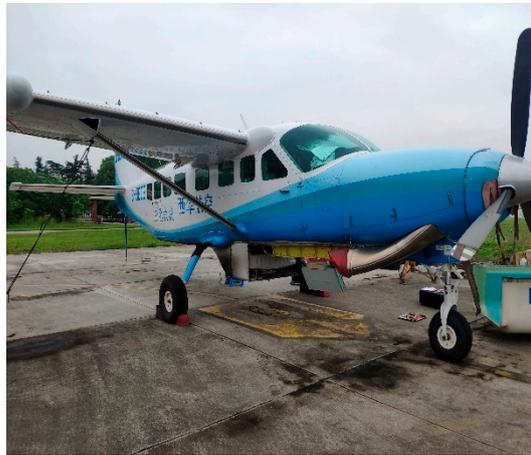
**Figure 5.** X/P-SAR system installed on Cessna 208.
