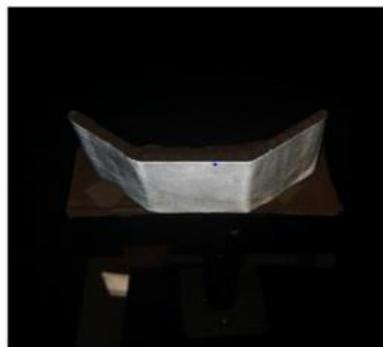
**Figure 5.** Planer combination target with retroreflective material.
