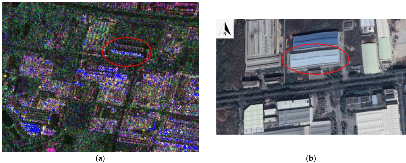
Figure 6. The 180-degree phase ambiguity determination process based on a specific building of this scene: (a) The local area of Figure 5b in the Jiangmen scene, the RDBs marked in blue triangles correspond to the left peak in Figure 5e, and the building circled in red is the target. (b) The optical image of the corresponding building on a Google image.
