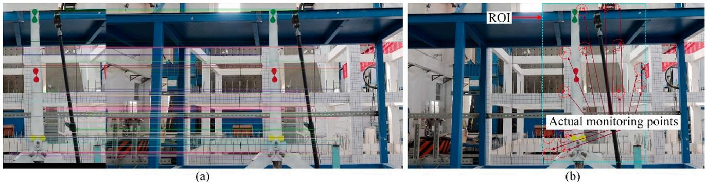
**Figure 16.** Monitoring effect of optical flow method in a complex background situation: (a) Harris corner matching in ROI area; (b) actual monitoring effect of optical flow method in ROI area.
