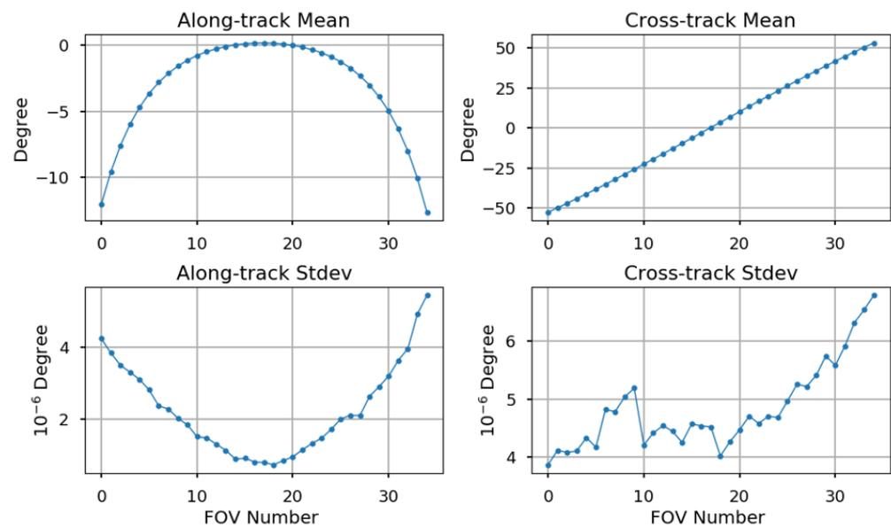
**Figure 7.** The along-track (left) and cross-track (right) angles in the S/C coordinate computed for the granule shown in Figure 1a, which contains 150 scanlines. The mean and standard deviations are given at the top and bottom, respectively.
