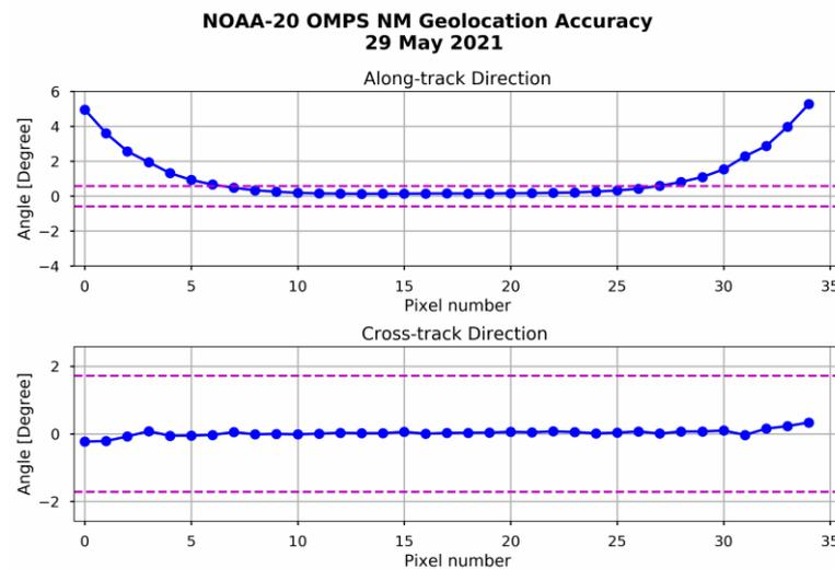
**Figure 11.** Geolocation assessment results, including the offset angles in the along-track and cross-track directions, where the dashed lines indicate the  $\pm 1/2$  macropixel FOV size in terms of degrees.
