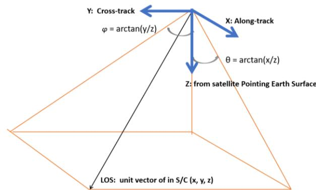
**Figure 6.** The OMPS LOS vector is expressed in the spacecraft coordinate, where the along-track ( $x$ - $z$  plane) and cross-track planes ( $y$ - $z$  plane) are formed. Two angles of  $\theta$  and  $\varphi$  simultaneously correspond to the unit vector of LOS.
