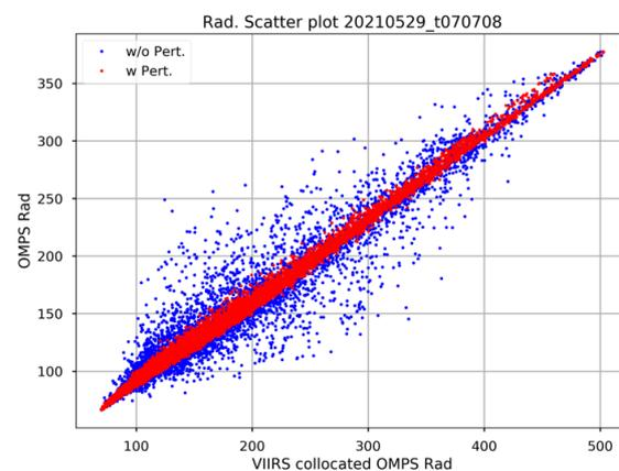
**Figure 5.** Scatter plot between real and VIIRS-collocated OMPS-NM radiances. The blue dots indicate the VIIRS-collocated OMPS-NM radiances using the original OMPS geolocation fields, while the red dots are perfectly aligned with the VIIRS. The radiance unit is  $W/(cm^3 Sr)$ .
