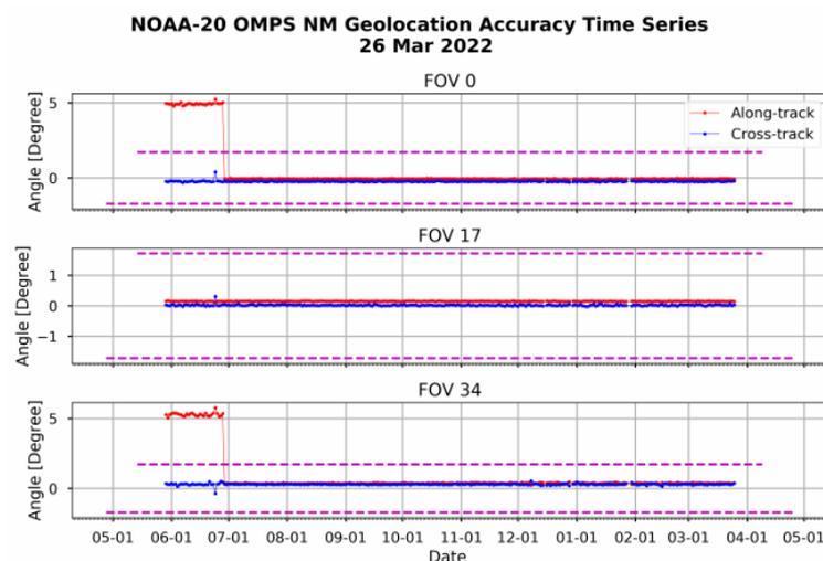
**Figure 13.** Time series of the assessment results for NOAA-20 OMPS-NM at macropixel FOV 0, 17 and 25, where different  $y$ -axis scales are used for three plots. The dashed lines indicate the  $\pm 1/2$  FOV size in terms of degree. The time series extended from 27 May 2021 to 26 March 2022 (309 days) and the data in each day contains 150–200 OMPS-NM lines with randomly selected non-uniform scenes.
