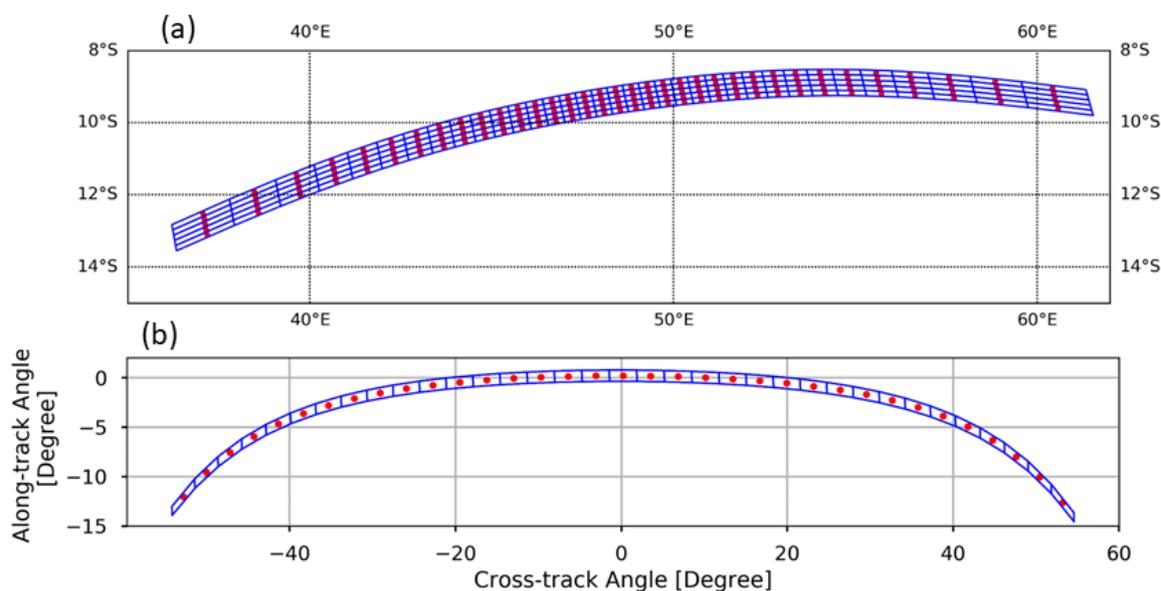
**Figure 3.** Example of OMPS-NM macropixel FOV shapes projected (a) on the Earth Surface, shown as longitude and latitude and (b) on the S/C coordinate expressed in the along-track and in-track angles (indicated by the bluesines). The red dots point to the FOV center. The FOVs on the Earth’s location in five scanlines return to identical locations on the S/C coordinate after the inverse geolocation computation.
