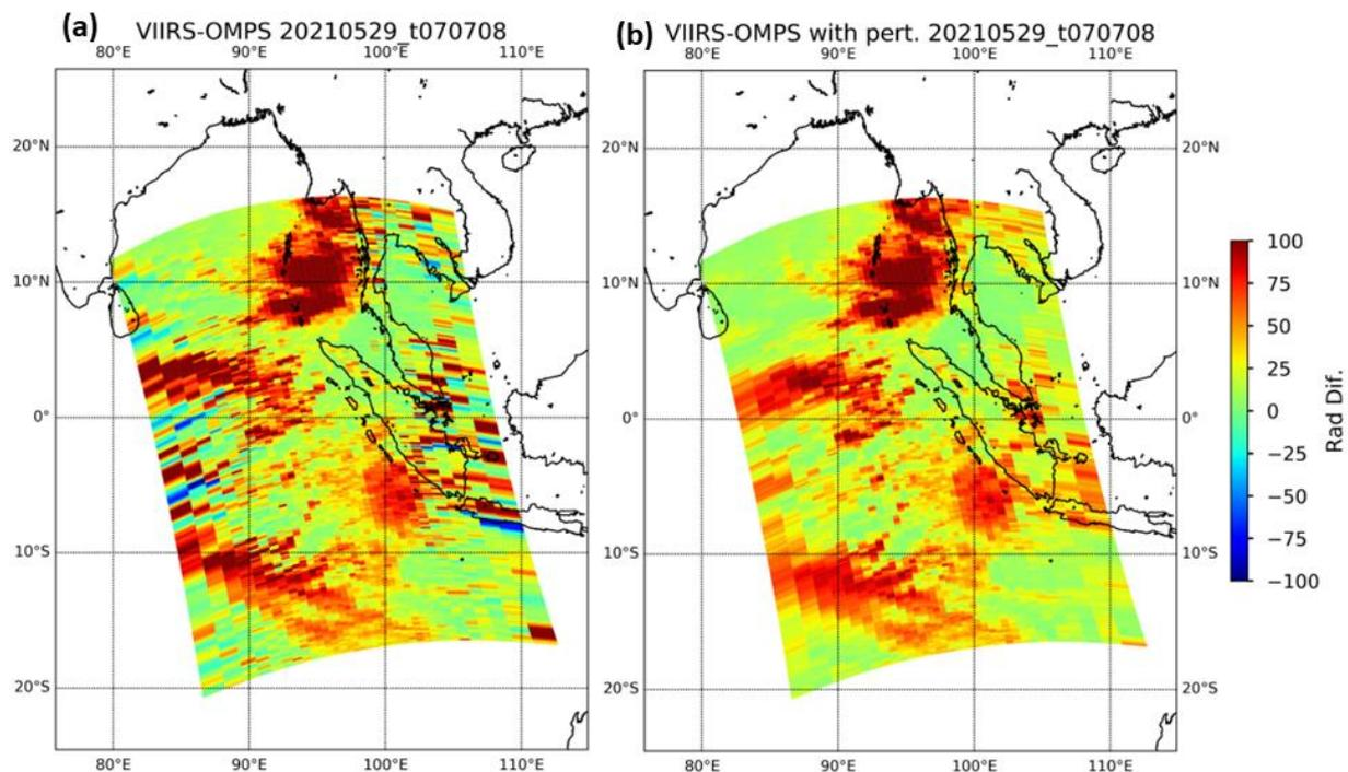
**Figure 4.** Radiance difference image between real and VIIRS-collocated OMPS-NM radiances: (a) based on the original OMPS geolocation fields and (b) the ones with perturbation that perfectly are aligned with VIIRS. The radiance unit is  $W/(cm^3 Sr)$ .
