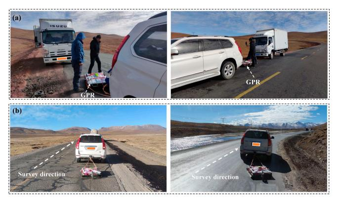
Figure 6. Diagram of the field GPR survey on QTH: (a) GPR survey system; (b) site survey.
