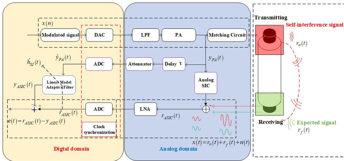
Figure 1. IBFD-UWAC system SIC model.
