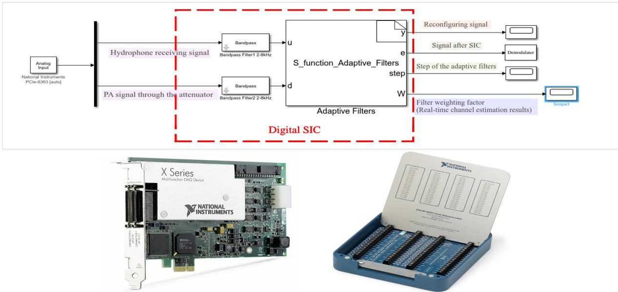
**Figure 4.** The top is Simulink<sup>®</sup> program block diagram and the bottom is PCIe-6363 device and NI SCB-68A Terminal Block, respectively.
