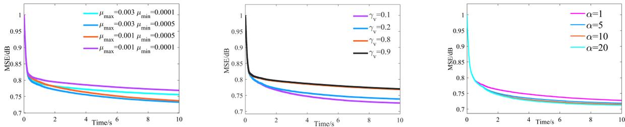
**Figure 5.** The MSE curves of the IVSS-LMS algorithm with different parameters. Left shows the MSE curves of the IVSS-LMS algorithm with different step-size, middle shows the MSE curves of the IVSS-LMS algorithm with different  $\gamma_v$  and right shows the MSE curves of the IVSS-LMS algorithm with different  $\alpha$ .
