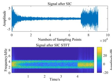
Figure 15. Time-frequency diagram of the signal after SIC.
