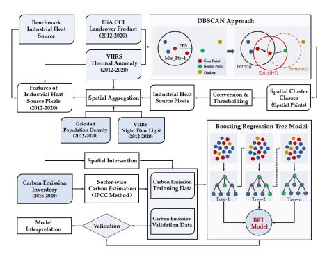
Figure 4. Flowchart of the data processing and modeling methodology utilized in this study.
