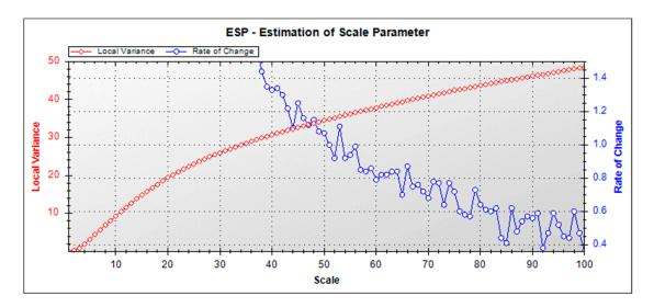
**Figure 4.** Local variance and rate of change of different values of scale calculated by the ESP tool with a shape of 0.1 and compactness of 0.5.
