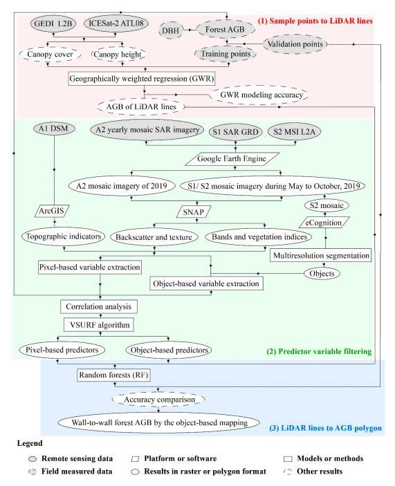
**Figure 2.** Overall workflow of object-based mapping of forest AGB by integrating LiDAR data with MSI and SAR images.
