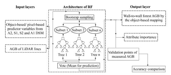
**Figure 5.** Delineation of random forests (RF) mapping of forest AGB based on LiDAR lines and multi-sensor images.
