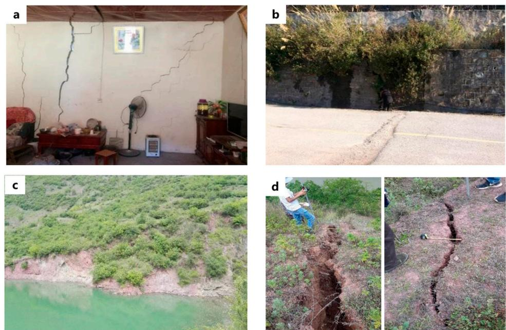
**Figure 2.** Field investigation of the Cheyiping landslide: (a) Damaged house; (b) Cracks in the road pavement; (c) Collapse of the reservoir bank; (d) Tensile cracks.
