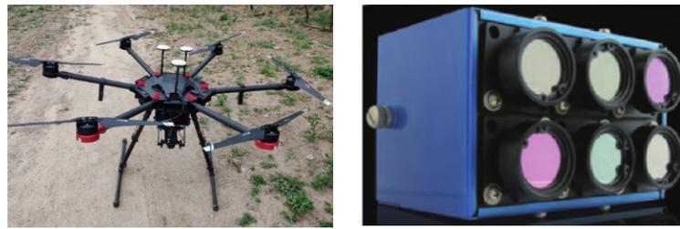
**Figure 1.** M600 UAV and Micro-MCA multispectral camera.
