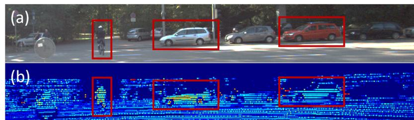
**Figure 5.** Visualization of (a) RGB image and (b) LiDAR intensity. Observing the red bounding boxes, the objects with higher LiDAR intensity have the clearer structural features in both RGB image and LiDAR point cloud.
