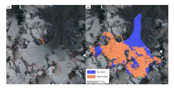
**Figure 12.** Abramov Glacier snow and ice classification, and SLA calculation. (a) Landsat image for Abramov Glacier in the NIR band, with some cloud cover and shadow affects. (b) Snow and ice classification for Abramov Glacier. Some misclassifications are marked by red circles; however, the SLA is unaffected. Orange arrows in (a,b) indicate the correct SLA calculations.
