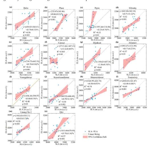
**Figure 9.** SLA–ELA relationships for the 14 reference glaciers. Blue points are the maximum SLA–annual ELA pairs, solid lines indicate the linear fits to the data, and red areas are the 95% confidence belts. Subfigures (**a–n**) represent the comparison of the relationship between the SLA and ELA of each glacier, respectively. The linear function equation in each subfigure is a linear fit equation.  $R^2$  and p are two values to assess the relationship and significance between SLA and ELA.
