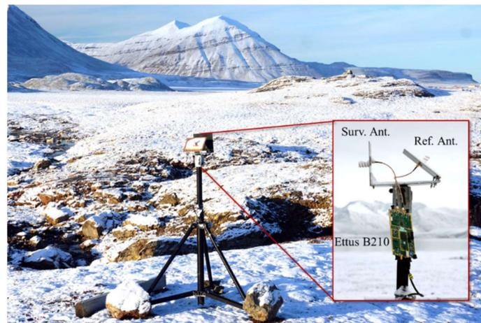
**Figure 17.** Setup of the experiment conducted in Spitsbergen, Norway. The system is fixed on the same position for a period of 12 days to show its stability and repeatability.
