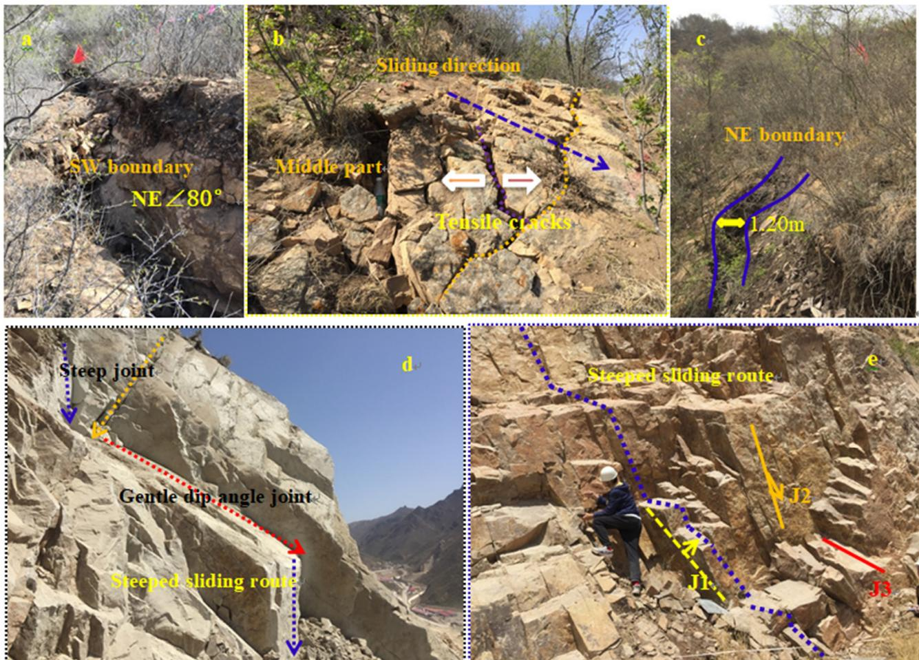
**Figure 15.** Composition and failure type of sliding failure surfaces (combination of stepped-gentle joints). Combination of stepped-gentle joints of sliding failure surface. (a) tension fissure at trailing edge. (b) tensile cracks in middle part. (c) shear fissure at NE boundary. (d) Combination of anti-inclined joint and inclined unloading joint. (e) Combination of inclined joint and inclined unloading joint.
