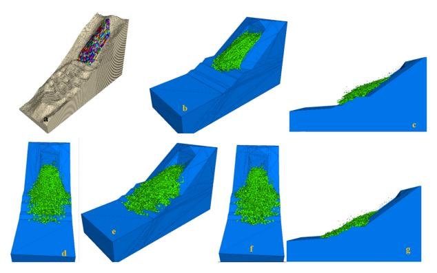
**Figure 13.** Influence range of landslide mass at different calculation time steps. (a) Numerical model. (b) T = 10,000. (c) T = 13,000. (d) T = 16,000. (e) T = 19,000. (f) T = 22,000. (g) T = 28,000.
