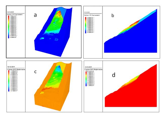
**Figure 12.** Displacement distribution in 10,000 steps of iteration. (a) Overall displacement distribution of YII4-3. (b) Displacement distribution at different elevations of YII4-3. (c) Overall displacement distribution of YII5-1. (d) Displacement distribution at different elevations of YII5-1.
