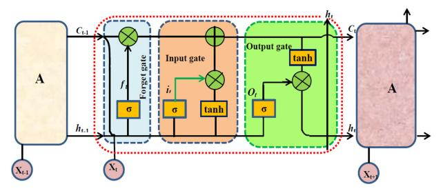
Figure 4. Main LSTM structure input and output.
