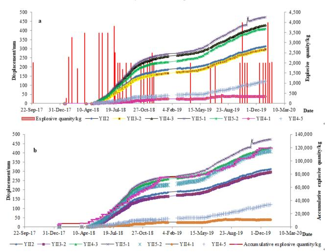
**Figure 9.** Explosive blasting and landslide displacement monitoring data: (a) displacement with daily blasting and (b) displacement with cumulative blasting.
