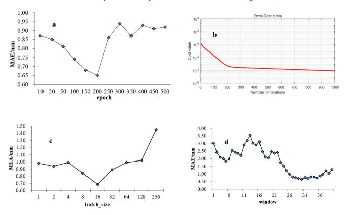
**Figure 17.** Influence of super parameters on LSTM model errors. (a) different epochs with MAE. (b) error cost with number of iterations. (c) different batch\_size with MAE and (d) different window with MAR.
