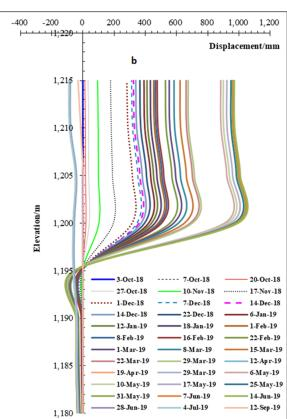
**Figure 7.** Process curve of deep displacement fixed inclinometers: (a) Monitor station CX03 and (b) Monitor station CX01.
