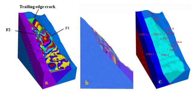
**Figure 11.** Numerical model of the excavated slope. (a) Numerical model. (b) Calculation section. (c) Monitoring points.
