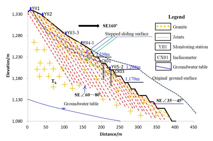
Figure 2. Stratigraphic profile of the cut-slope.
