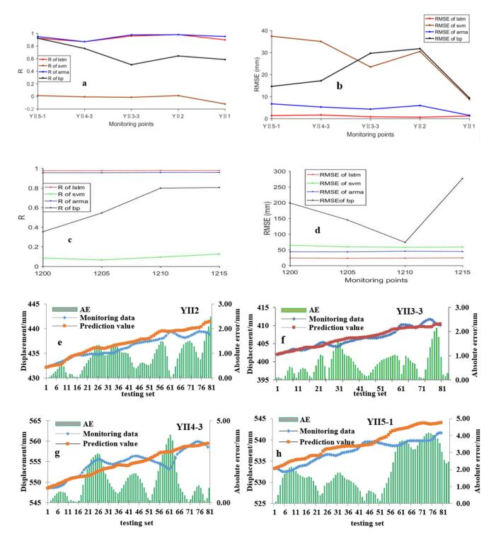
**Figure 16.** Accuracy evaluation of the different model forecasts. (a) Regression coefficient R of surface displacement. (b). Root mean square error RMSE of surface displacement. (c). Regression coefficient R of different inclinometer. (d). Root mean square error RMSE of different inclinometer. (e–h) absolute error of LSTM model of different monitor stations.
