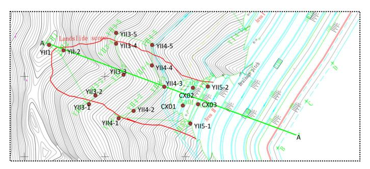
Figure 3. Layout of landslide monitoring points.
