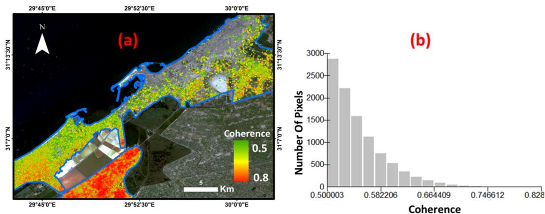
**Figure 11.** The final coherence coverage of ALOS-2 data which is very poor with average coherence values of about 0.6, standard deviation of 0.04 and about 80% of Alexandria City show no coherent data (a) and its associated histogram (b).
