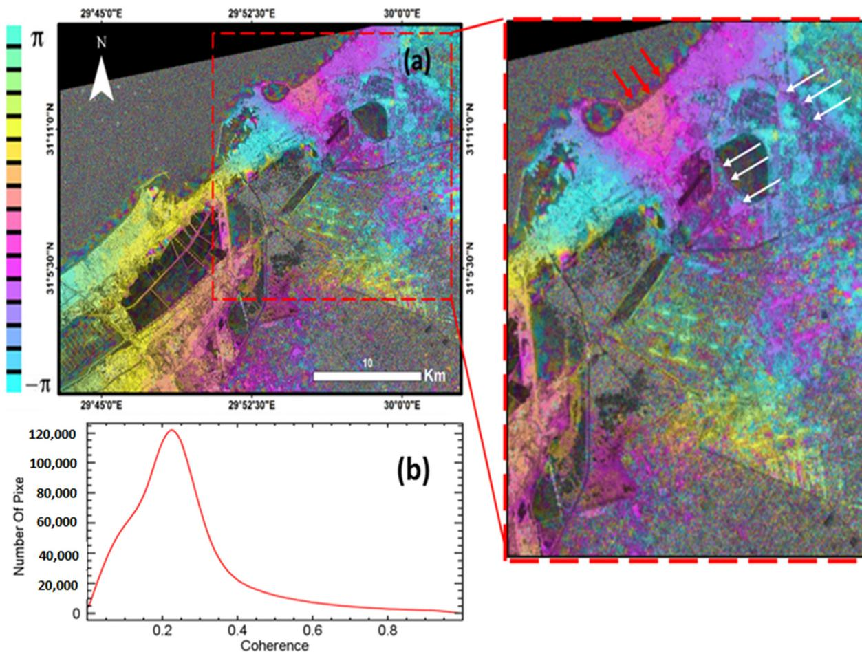
**Figure 6.** (a) Wrapped ALOS-2 low coherent interferogram showing errors during the flattening sub-step; white arrow indicates systematic residual fringes that could have been caused by strong orbital inaccuracy or issues with some parameter settings, while red arrows indicate strong atmospheric artifacts and phase jumps. (b) Histogram representing the coherence value of interferogram with a mean coherent value of 0.15.
