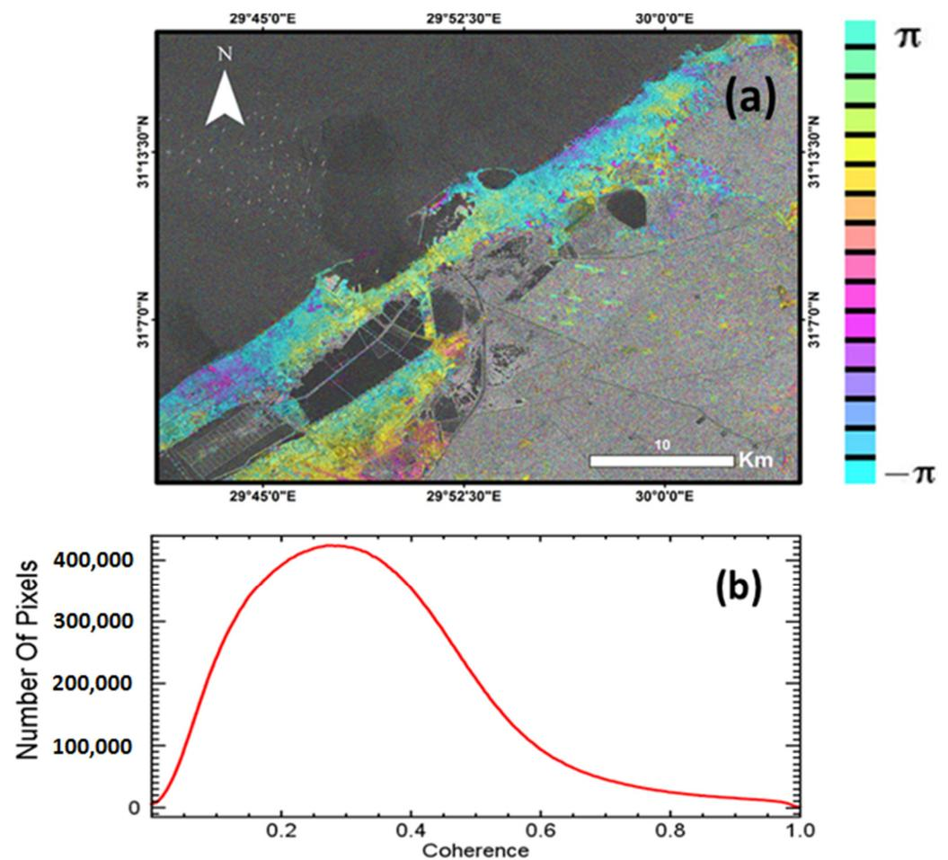
**Figure 7.** Wrapped Sentinel-1 interferogram with low coherence. The cause is the very large temporal and normal baseline between the two acquisitions used to make the interferogram (a). The histogram illustrates the coherence value between two interferogram pairs (master 15 December 2018 and Slave 10 June 2019) (b).
