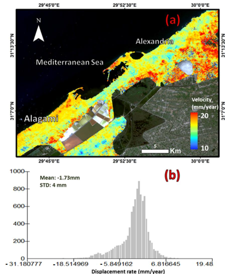
**Figure 14.** (a) The estimated mean displacement velocity of Alexandria and Alagami Cities using the Sentinel-1 data from August 2017 to September 2020 with coherence threshold of 0.4; (b) the corresponding histogram distribution of the derived displacement velocity rates.
