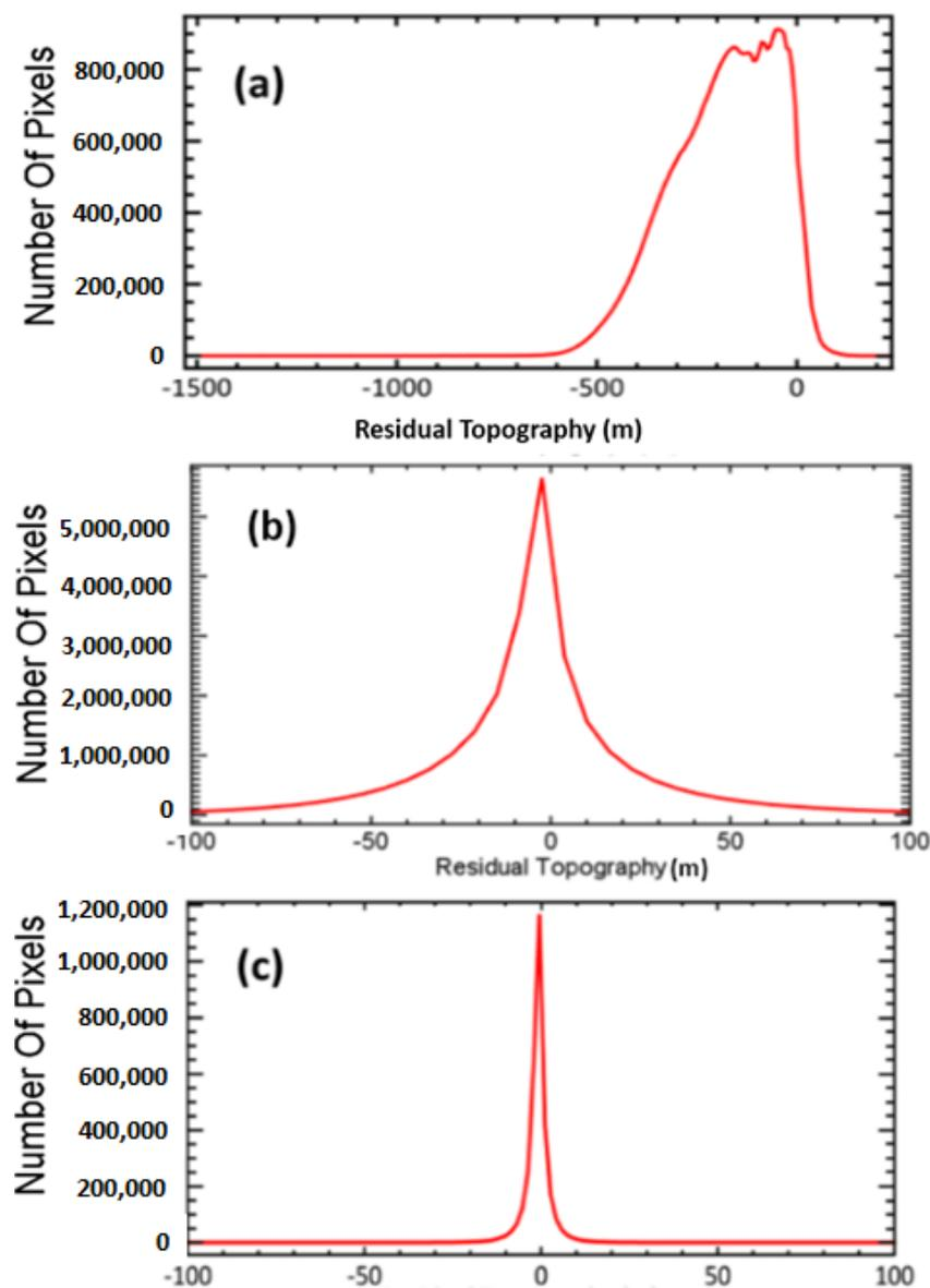
**Figure 8.** Statistics of estimated residual topography: (a) for ALOS-2 interferograms by using the SRTM data, which showed average residual topography equal to  $-100$  m and high standard deviation equal to  $70$  m; (b) the average residual topography and standard deviation reduced by increasing the wavelet number; (c) for Sentinel-1 interferogram with average residual topography to almost  $0$  m with a standard deviation equal to  $13.5$  m.
