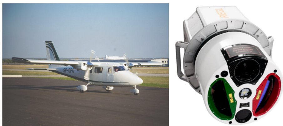
Figure 5. LiDAR Vulcanair P68C plane and VQ-1560i DW laser scanner, property of Opegieka Sp. z o.o.
