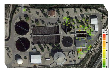
Figure 7. Map of H<sub>2</sub>S concentration obtained from drone measurements.
