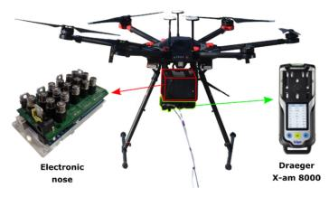
**Figure 2.** DJI Matrice 600 Pro drone equipped with a custom e-nose and a Dräger X-am 8000 analyzer. The inlets of both systems are connected to 10-m PTFE tubing.
