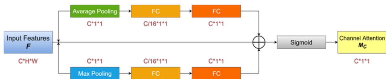
Figure 3. Basic framework structure of the channel attention module.
